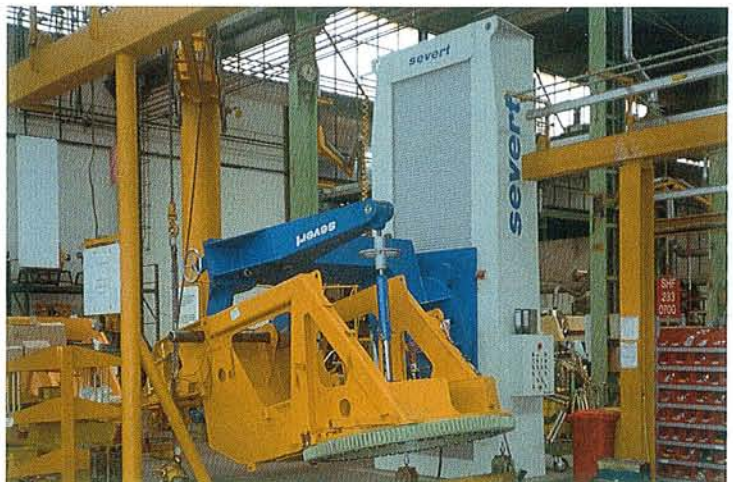
Application at a construction machine manufacturer component weight 13000 kg
