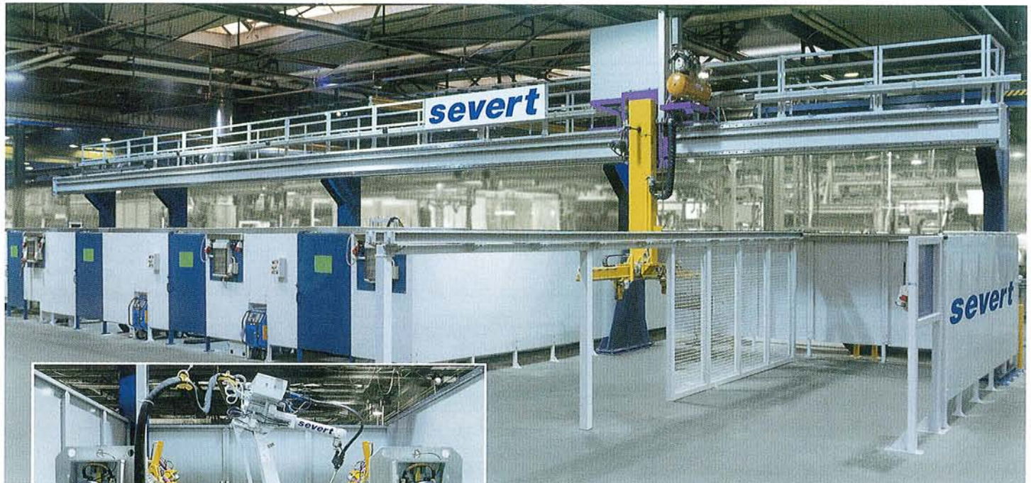
Production line with robot-cells and automated component transport for welding and cutting vehicle components.
